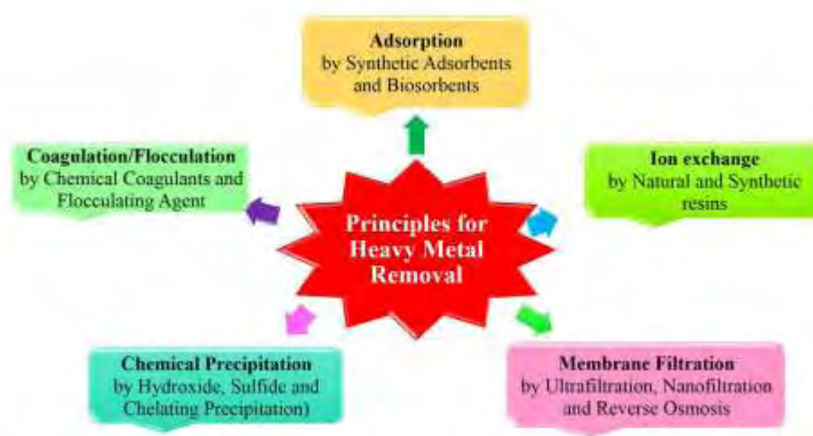
Figure 2 Basic principle of different methods for heavy metal removal 32
