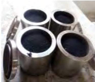
Conversion of bone waste into bonechar and then nano bone char through ball milling technique
