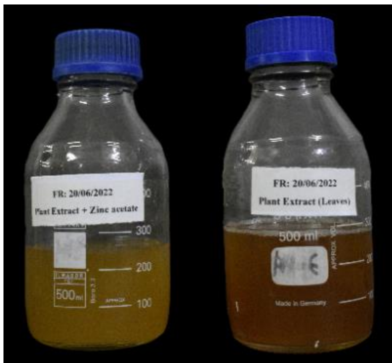
Figure 4.2. Biosynthesis of ZnO NPs from extract of Picea smithiana by using Zinc acetate.
