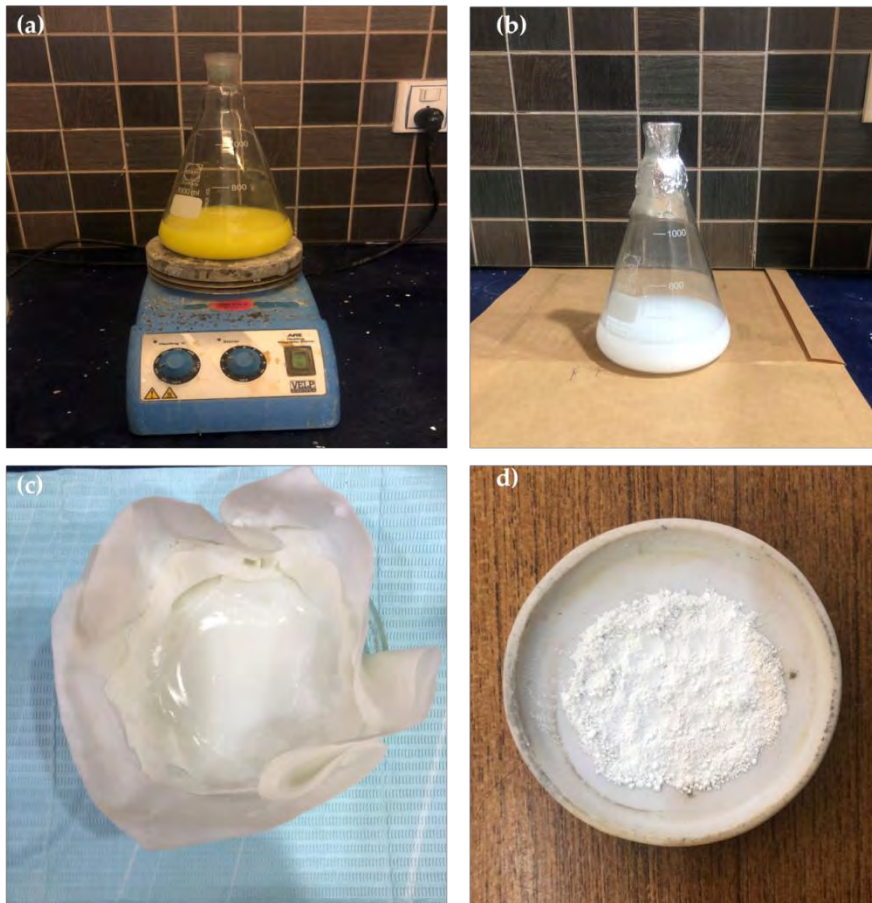
Figure-4.1: Synthesis of Titania ( \text{TiO}_2 -Nps) by Bacillus coagulans : (a) Bacillus coagulans culture solution, (b) Titania ( \text{TiO}_2 -Nps) in solution form, (c) Cake form of Titania ( \text{TiO}_2 -Nps) and (d) Fine powdered form of Titania ( \text{TiO}_2 -Nps).
