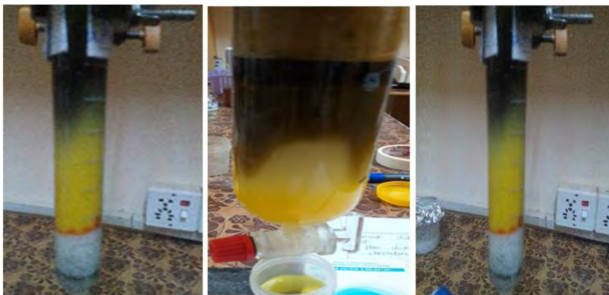
Figure 3.1. Different bands in packed column due to movement of mobile phases.
