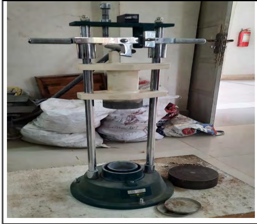
Fig 3.7 Aggregate Impact Value machine at SABHAN Geotechnical Laboratory.
