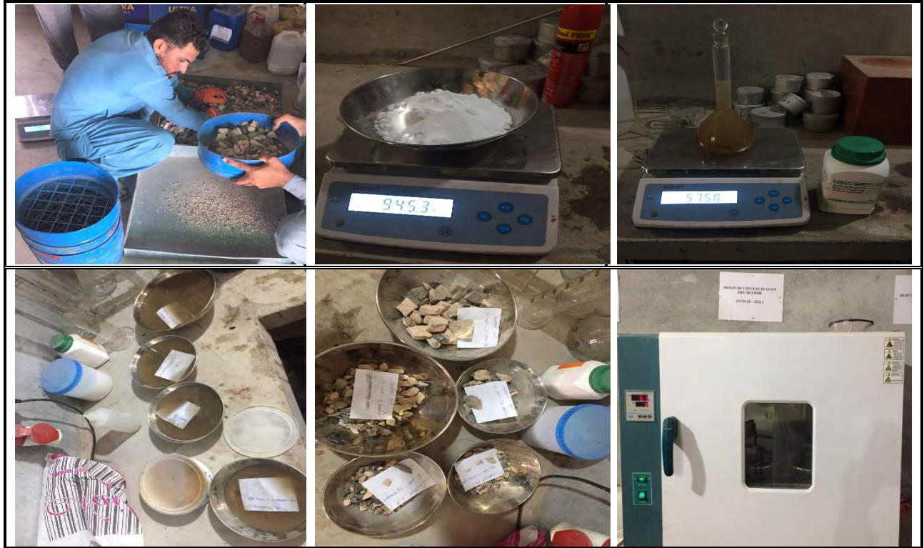
Fig 3.6 Soundness test in progress at SABHAN Geotechnical Laboratory.
