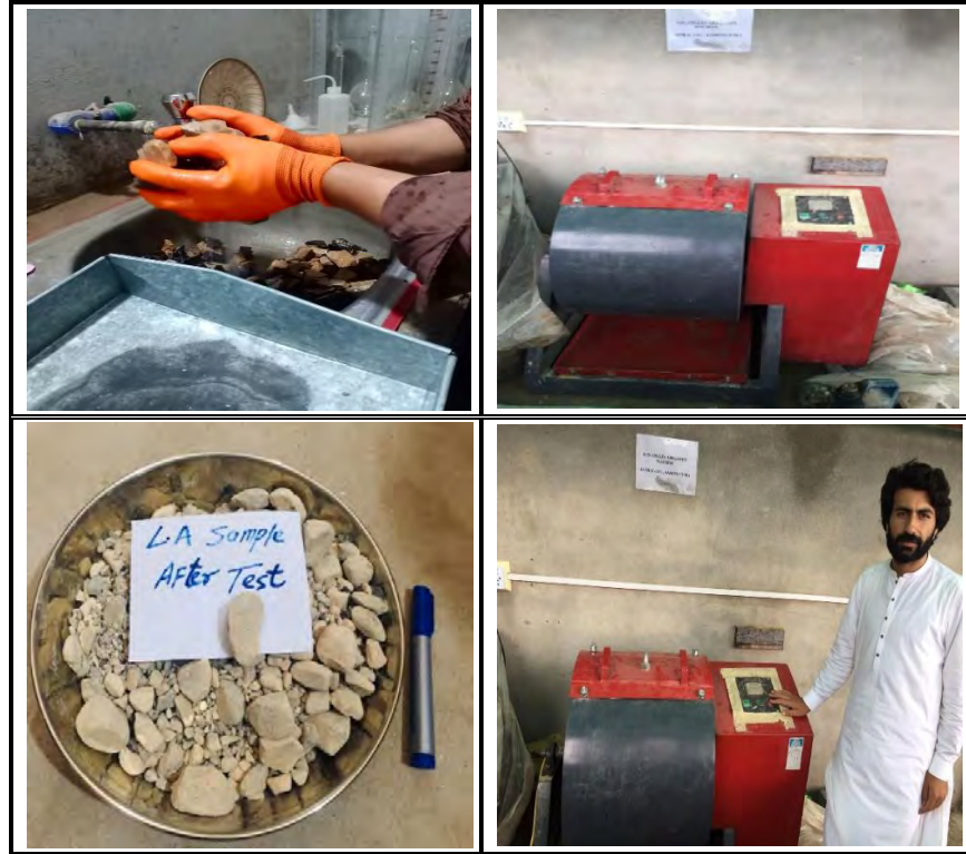
Fig 3.5 Loss Angeles abrasion test in progress at SABHAN Geotechnical Laboratory.
