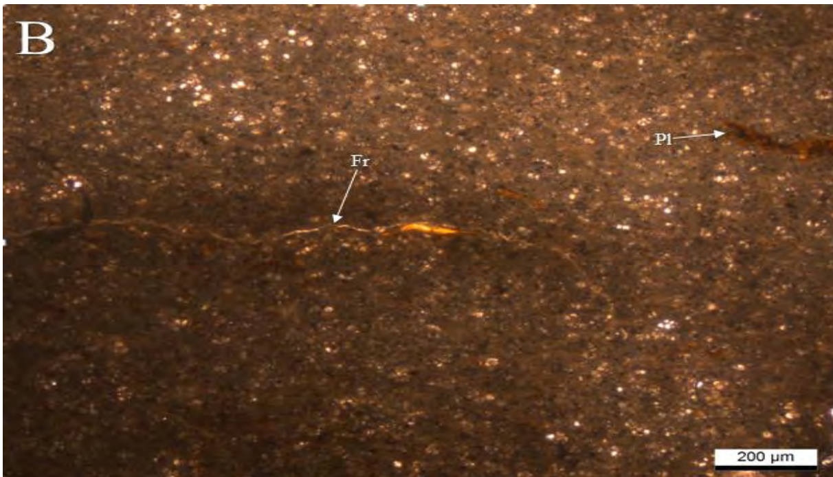
Fig 4.4 Photomicrograph of Habib Rahi Limestone (HR-2) showing Fracture (Fr), and Pyrite leaching (Pl).
