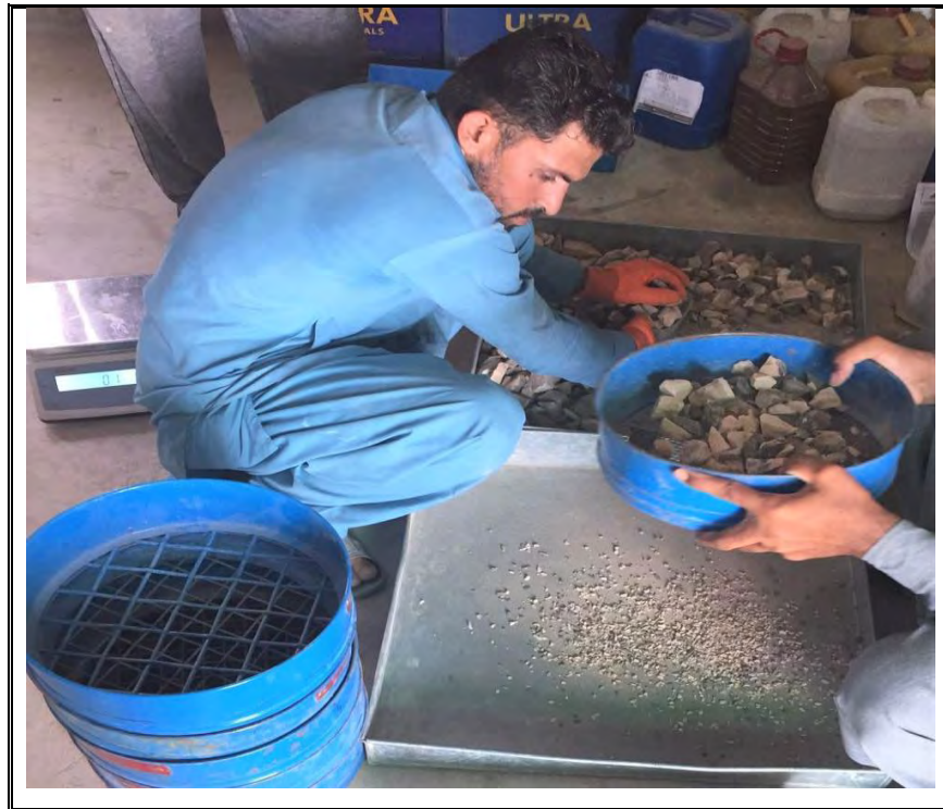
Fig 3.4 Sieve Analysis in progress at SABHAN Geotechnical Laboratory.
