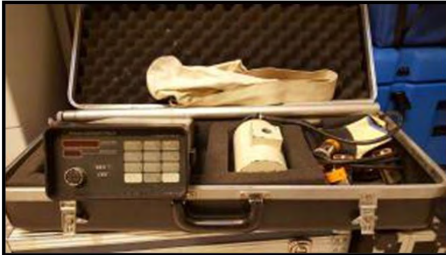
Figure 3.2: G-856AX Geometrics Proton Precision Magnetometer used for magnetic data acquisition.
