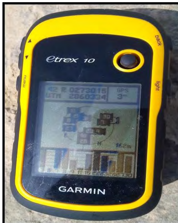
Figure 3.3: Garmin hand-held GPS used to determine the coordinates of the observation stations.
