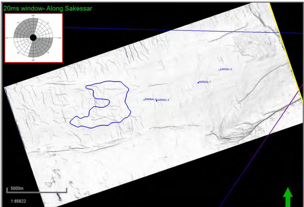
Figure 5.10: Ant track attribute of Eocene carbonate with dark lines of highly intense fracture zones in the inset conductive producing zones from Eocene carbonates are shown by tadpole. From Ant track trend, it is hence proved Karsal 01 & 03 are falling in fracture intense zones and Karsal-02 & 04 missing the fracture zones. Moreover, the generated probs results has also matched with Sakesar core of Talagang X-1. Table-3 shows different calculated parameters based on interpretation of azimuthal velocity analysis and ant tracking.
