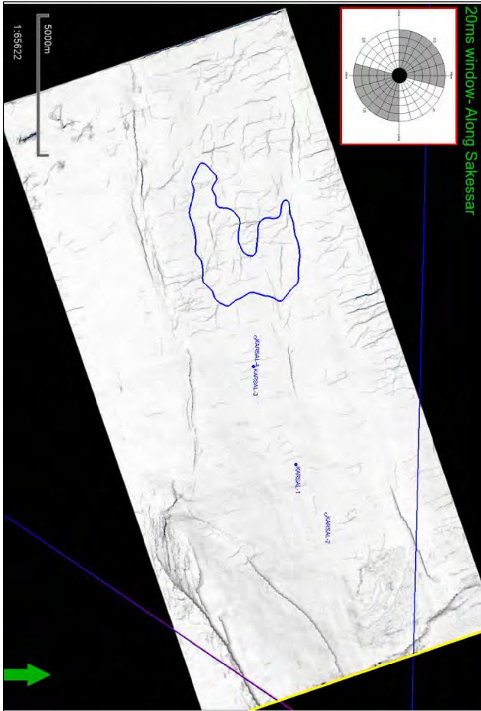
Figure 3.26: shows the ant track results from Petrel algorithm More Fractures at Karsal-3 (higher production) than Karsal-1 (less production). No Fractures at Karsal-2 and Karsal-4--- non-Producer. Good Fractures network are evident on Karsal Prospect as well along with karsal 1 and 3 together which give strength to move for drilling because minute trending lines represent the fracture corridor network not single line for one set of fracture.
