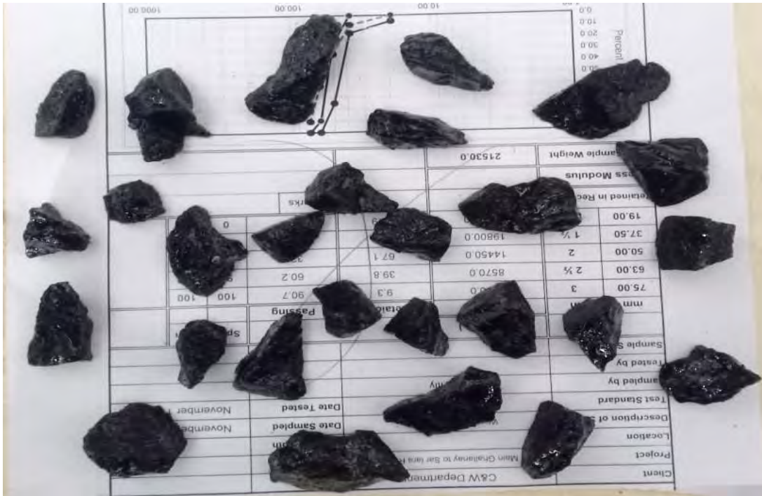
Figure 3.10 Showing Coating and stripping test of Kawagarh Formation conducted at Geotechnical Lab of National Engineering Services of Pakistan (NESPAK)
