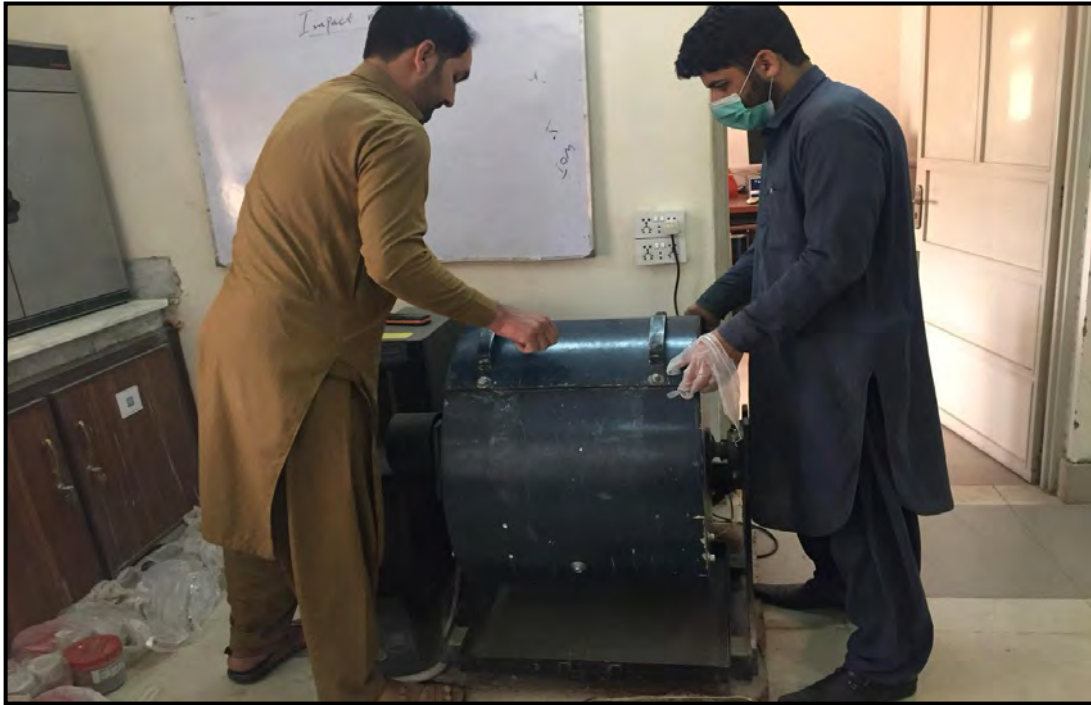
Figure 3.5 showing Los Angeles and abrasion equipment housed in Geotechnical Lab of NCEG
