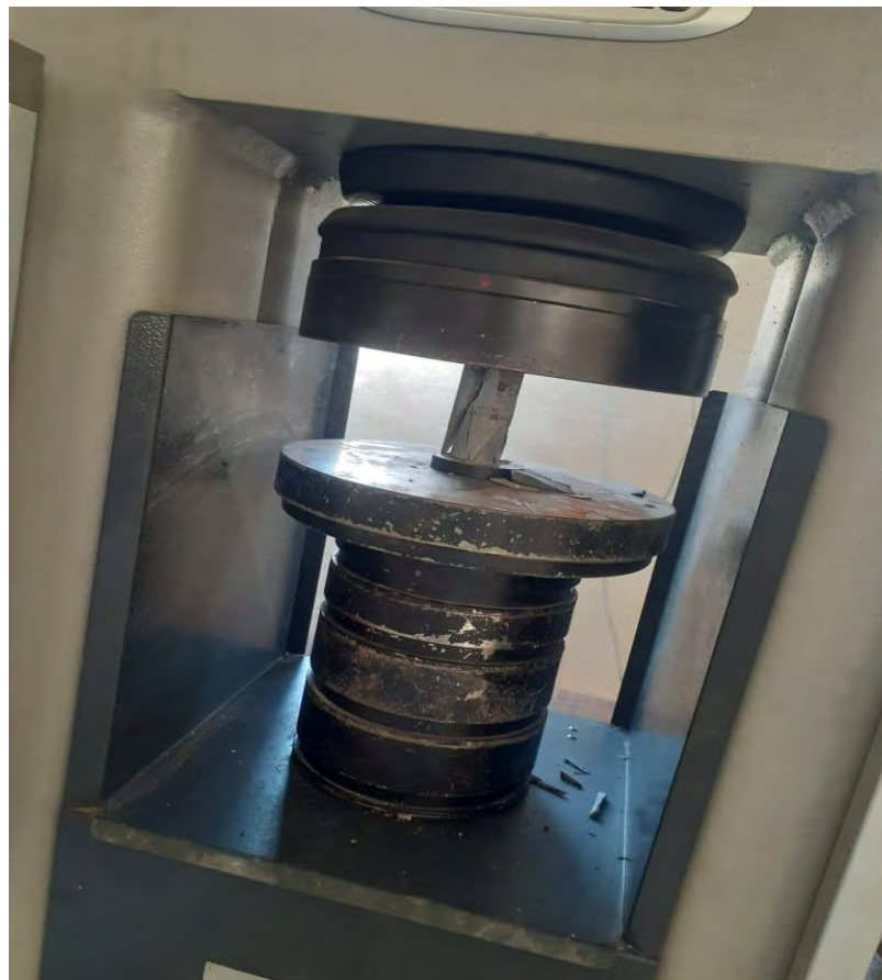
Figure 3.9 Photograph reflecting UCS test in progress.
