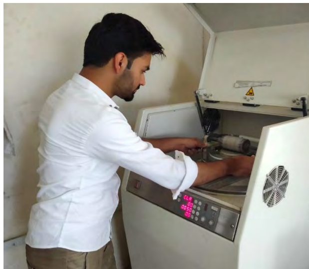
Figure 3.6 Powdering of rock samples in the tungsten carbide ball mill machine.
