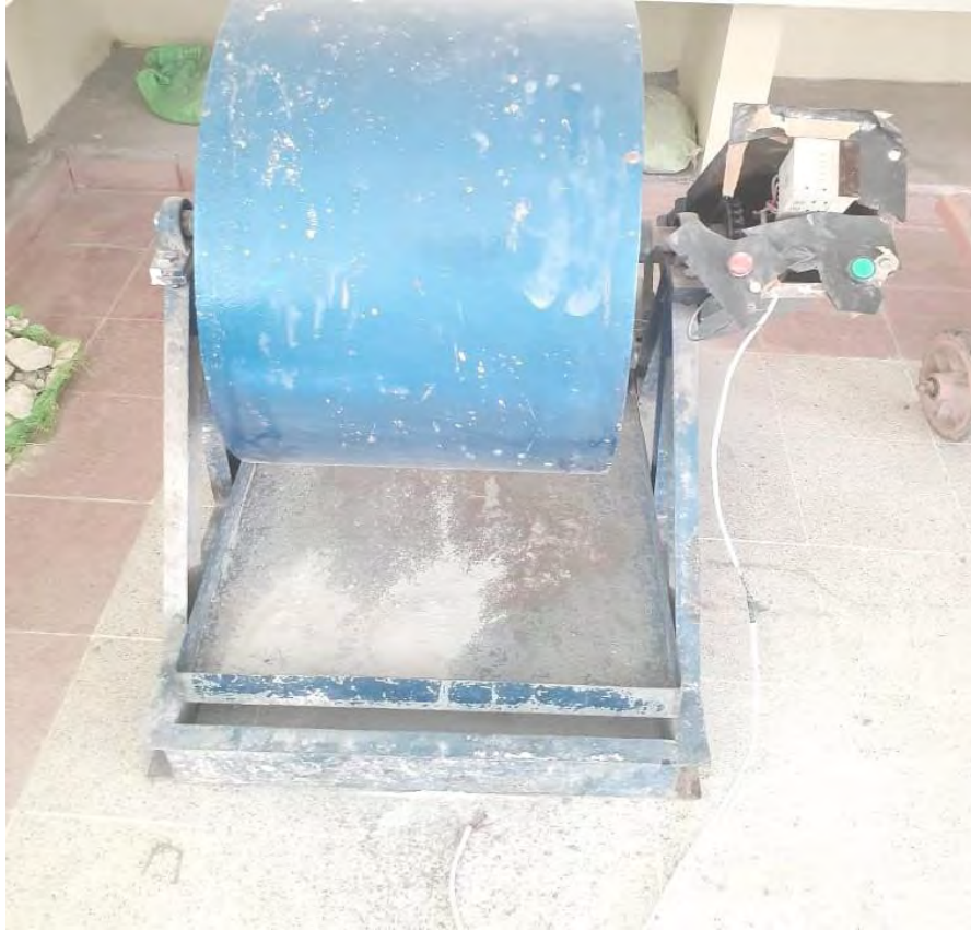
Figure 3.10 Showing Los Angeles and Abrasion test in Progress.
