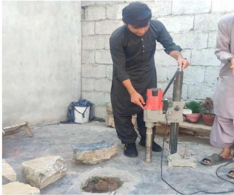
Figure 3.8 Coring of bulk samples in Progress.
