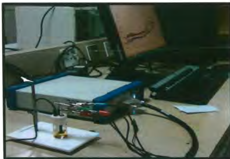
Figure 2.1 Electrochemical workstation connected with a voltammetric cell.
