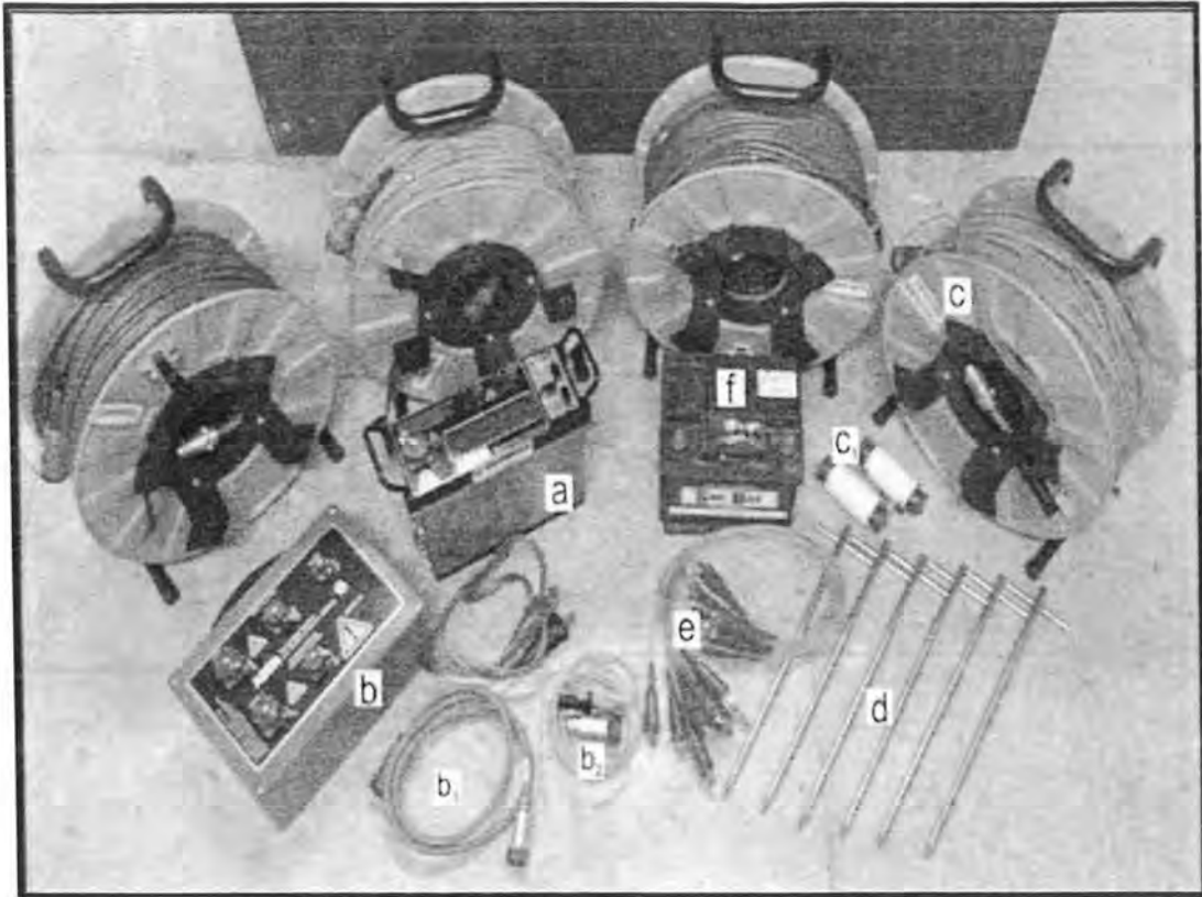
Fig.4.4Electrical resistivity method Equipment: (a) Terrameter SAS 4000, (b) selector and (b1 and b2) connectors, (c and c1) cable and connectors, (d)electrodes, (e) cable-electrode connectors and (f) battery supply.
