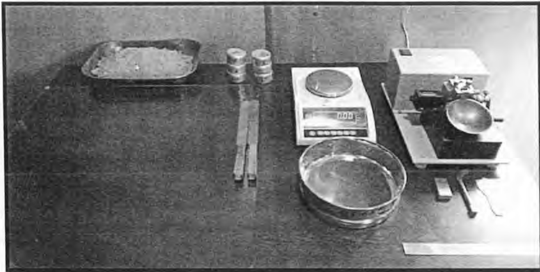
Fig. 4.6 Apparatus for liquid limit by Casagrande method.
