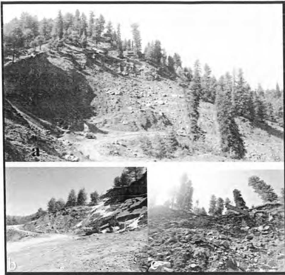
Fig.5.2a Main scarp of landslide., b -Main scarp at the head of the landslide near road, c -Fractured sandstone of the Murree Formation exposed at main scarp.
