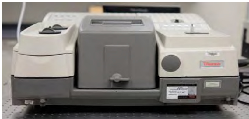
Fig 3.8: Thermo Nicolet 5700, Fourier Transform Infrared Spectrometer (FTIR)
