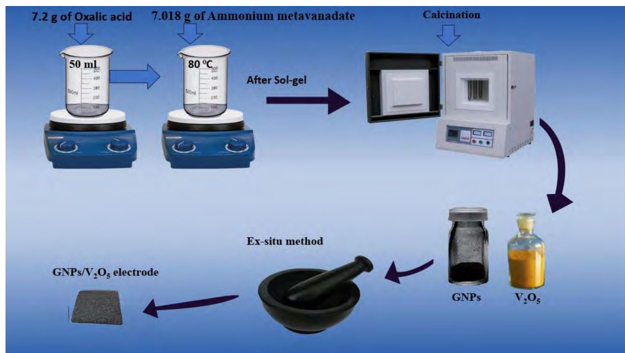
Figure 2.2: Synthesis flow chart of V_2O_5 nanostructure
