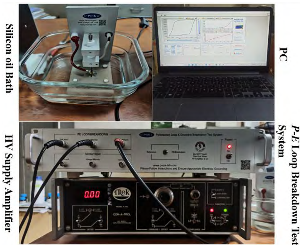
Figure 2.12 PolyK Polarization loop and Dielectric Breakdown Test System
