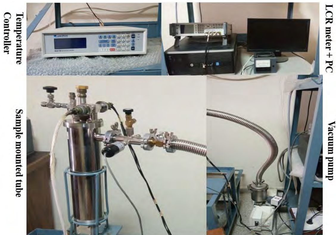
Figure 2.9 High temperature dielectric setup
