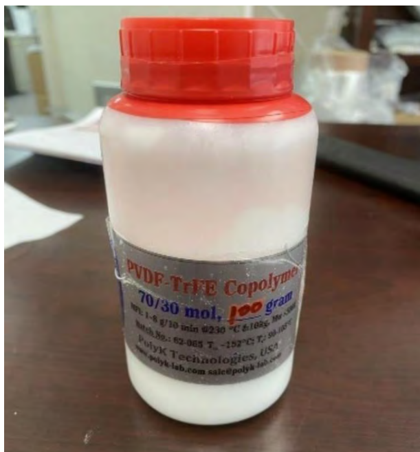
Figure 3.3 100-gram Resin of P(VDF-TrFE) 70/30 mol Copolymer [80]
