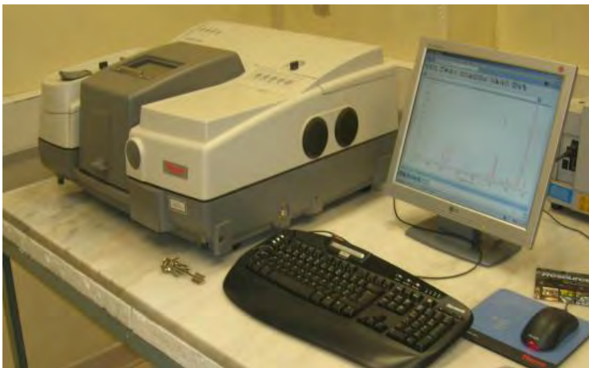
Figure 2.5 Nicolet 5700 FTIR Spectrometer [66]
