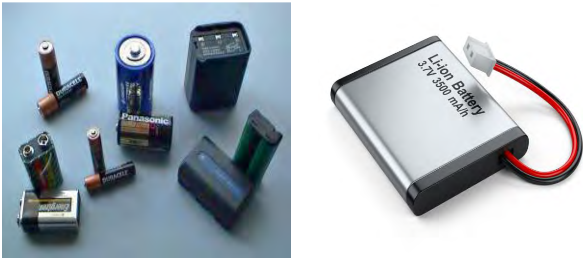
Figure 1.2 Primary batteries (Alkaline batteries, silver oxide batteries & secondary batteries (Lithium-ion battery) [10]
