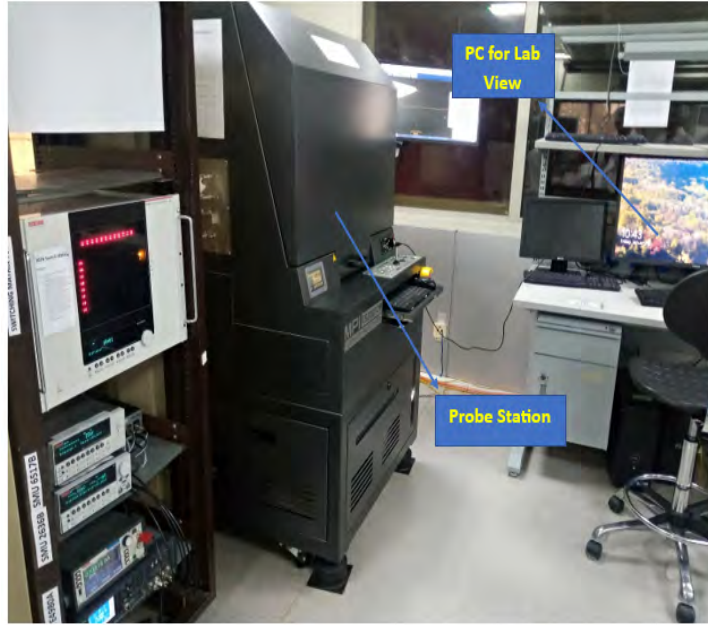
Figure 6.3: In the cleanroom at NCP, utilize the Probe System and PC running Lab VIEW.
