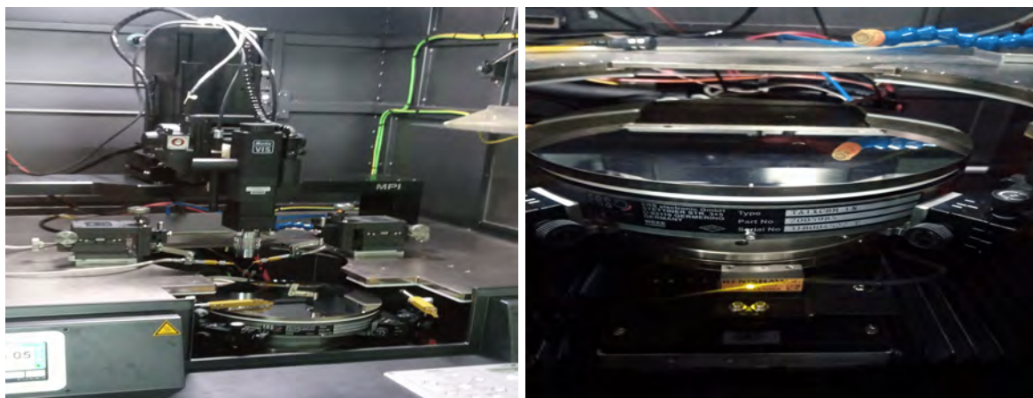
Figure 6.2: Functional Sensor Placement on Chuck vs. Optical Sensor Inspection
