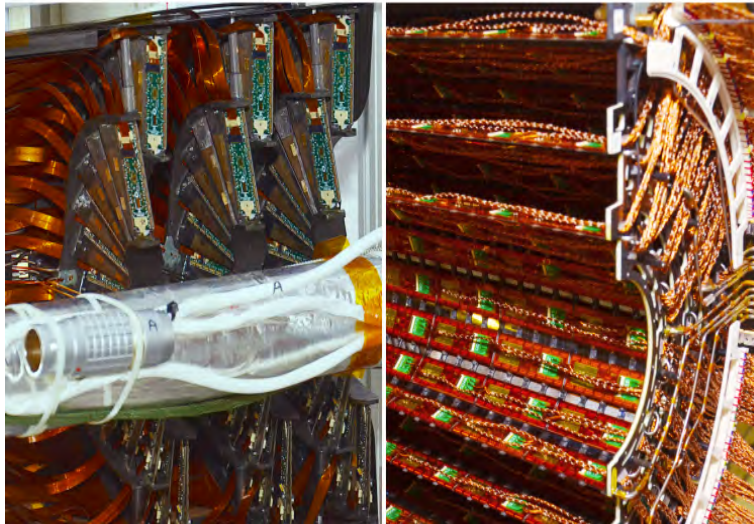
Figure 2.7: Schematic view of Silicon Pixel detector [11].
