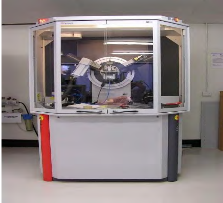
Figure 3.11: Pictorial diagram of X-Ray Diffraction Apparatus
