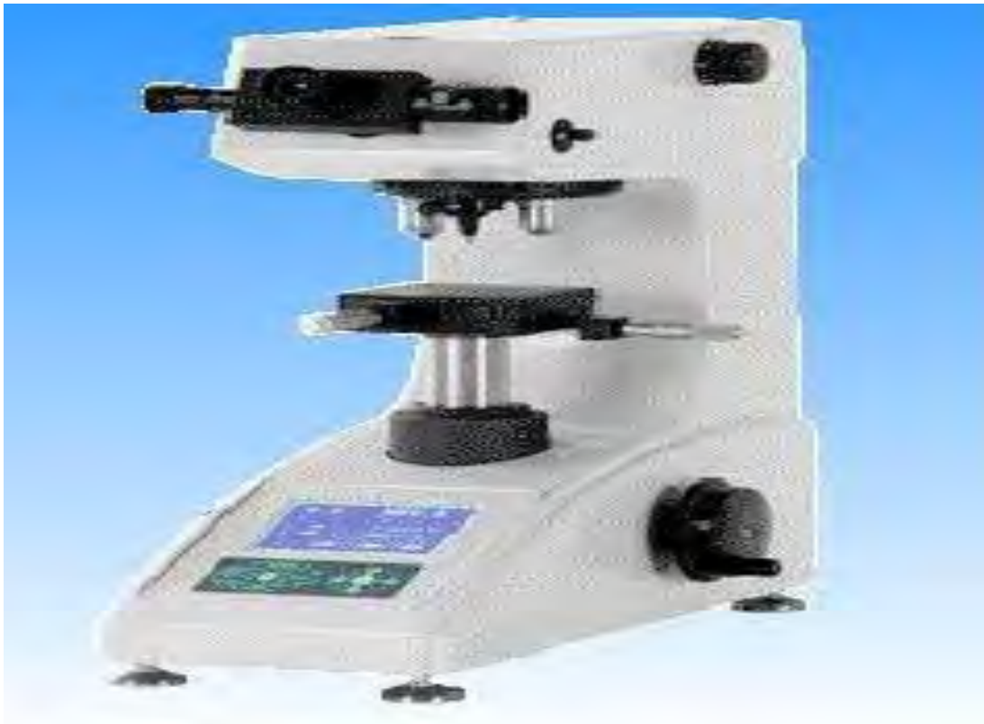
Figure 3.13: Pictorial diagram of Vickers hardness tester
