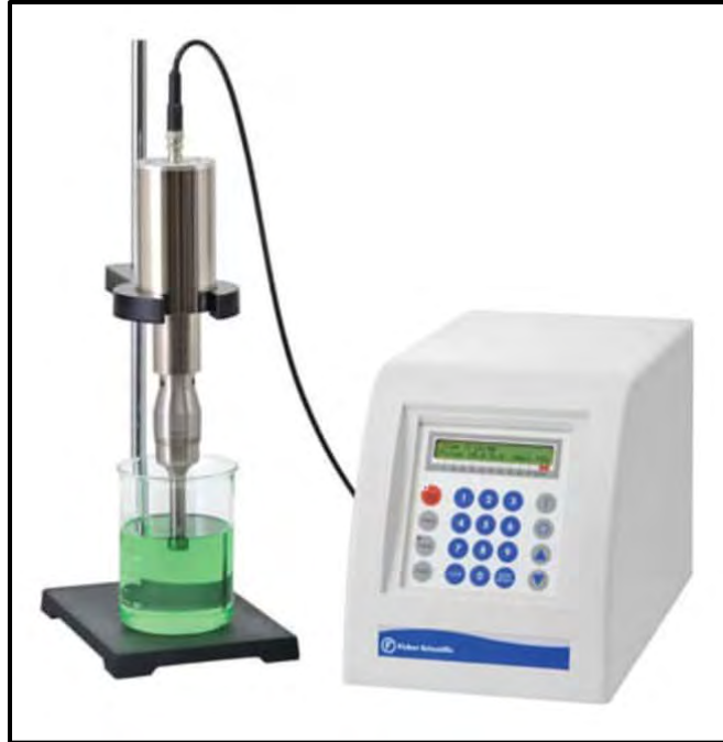
Figure 2.1: Sonicator for substrate washing.
