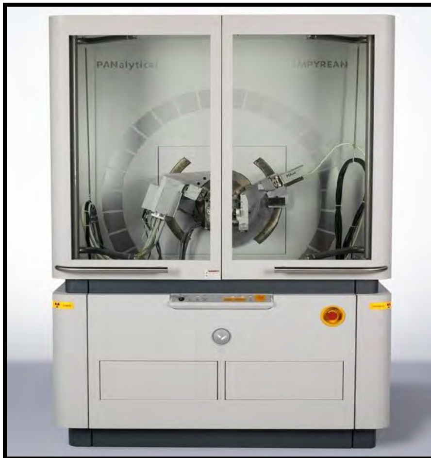
Figure 2.7: PAN analytical EMPYREAN X-ray Diffractometer.
