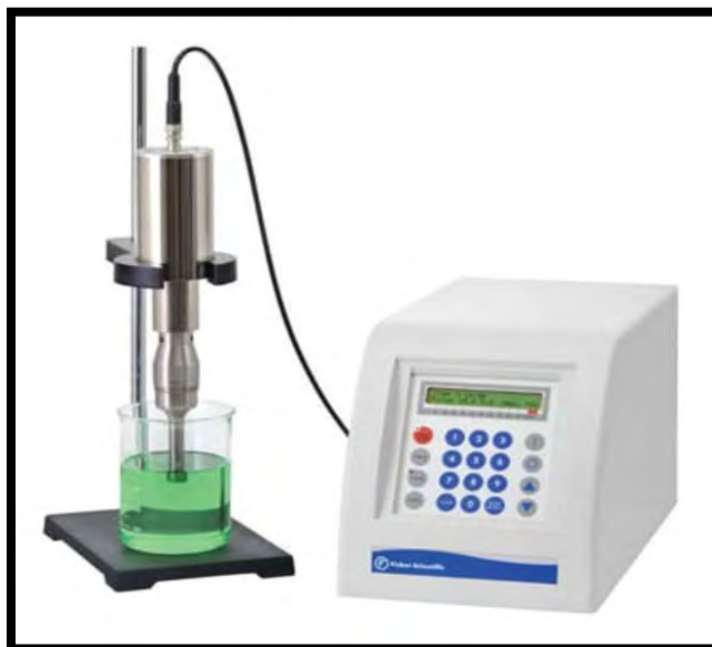
Figure 2.2: Sonicator used for substrates washing.
