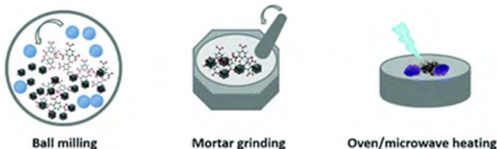
Figure 2.3: Schematic diagrams have been presented to illustrate the process of solvent-free synthesis of MOFs from solid materials[83]
