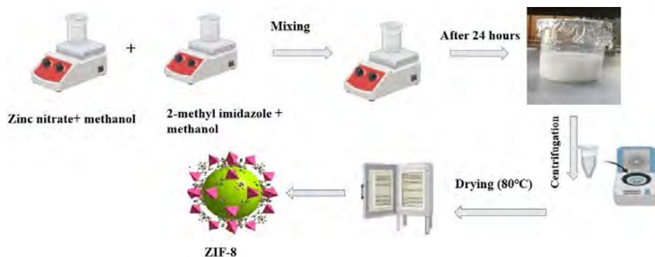
Figure 2.4: A pictorial representation of steps involved in the synthesis of ZIF-8
