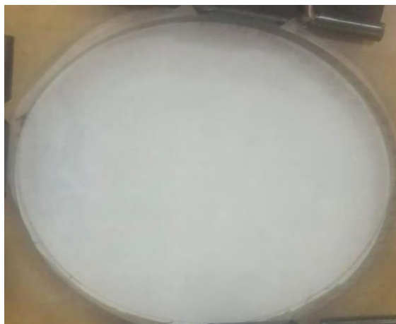
Figure 2.9 : Thin film composite-PA membrane
