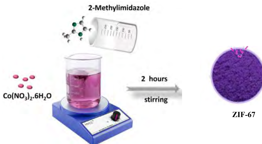
Figure 2:2: Procedure for synthesizing ZIF-67 [93]
