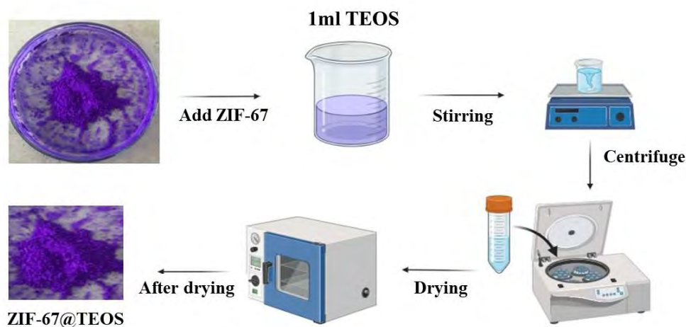
Figure 2:4: Procedure for synthesizing ZIF-67@TEOS
