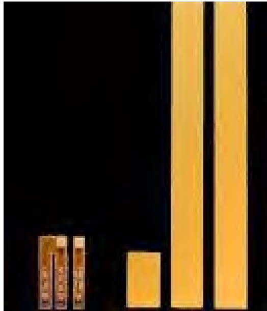
Figure 6.3.5: A set of Kapton strips (right) and HV tails for the top and bottom sensor (left).
