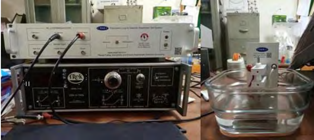
Figure 2.15 PolyK test systems for dielectric breakdown and polarization loop
