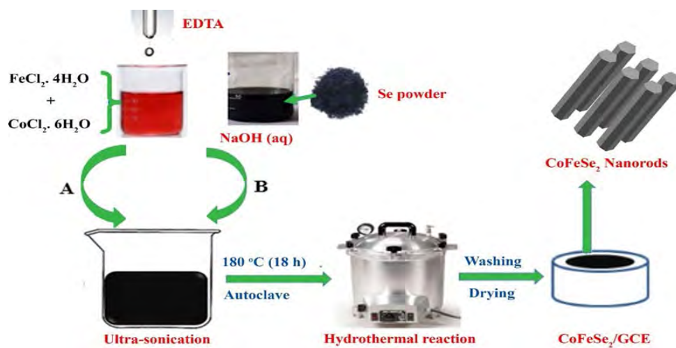
Scheme 2.3. A diagrammatic representation of the process for synthesizing FeCoSe_2 .
