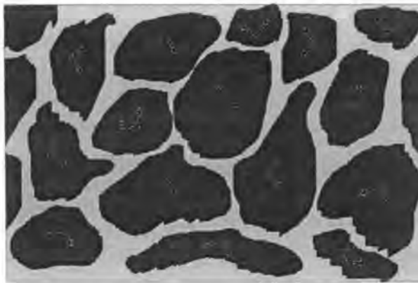
Fig 1.11 Schematics of the HTS microstructure: Differently oriented single crystal grains are separated by regions filled with secondary phases. In addition, oxygen depletion may occur at grain boundaries
