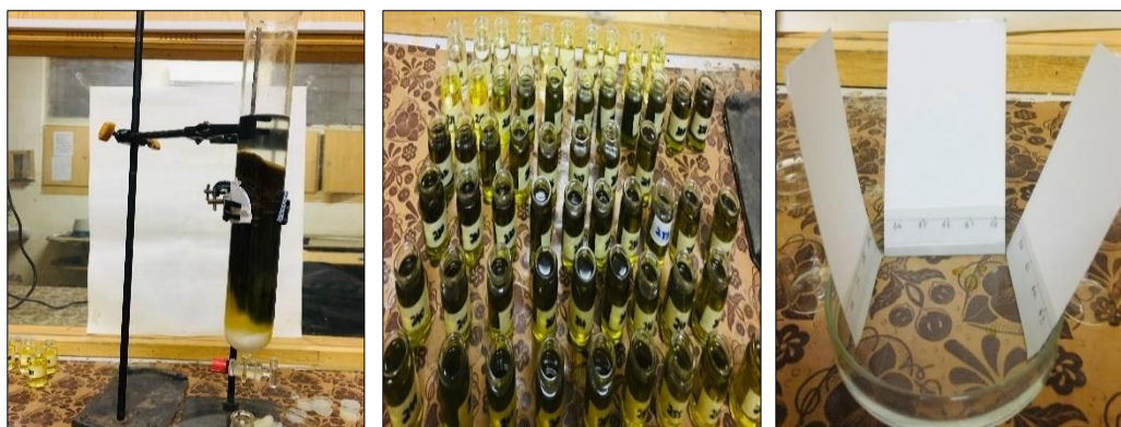
Figure 4.3(a): Fraction isolation by column chromatography, (b) Fractions obtained. (c): Thin layer chromatography of V. officinalis ' fractions
