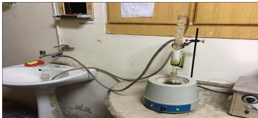
Figure 4.2: V. officinalis extract preparation in Soxhelt apparatus
