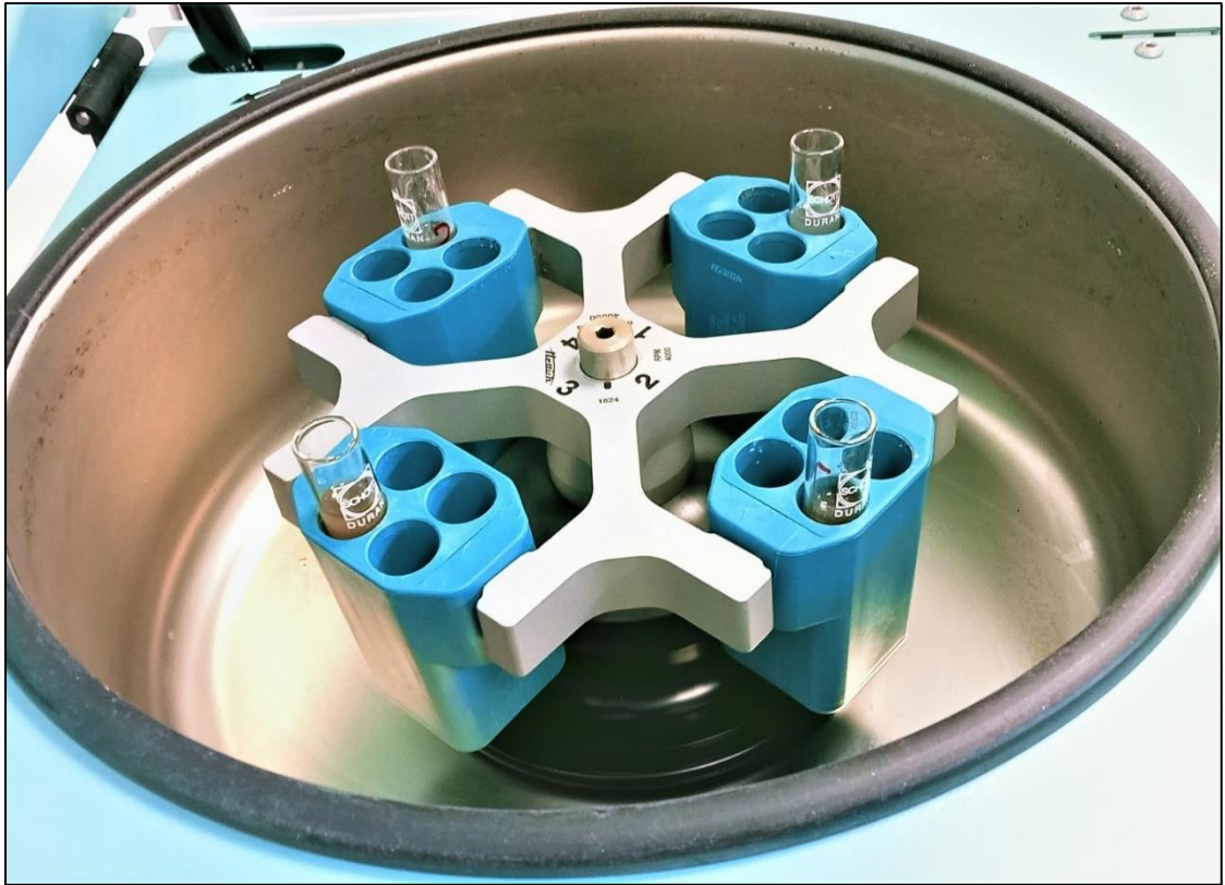
Plate 9. Centrifugation of the liquid samples to separate particles based on size.
