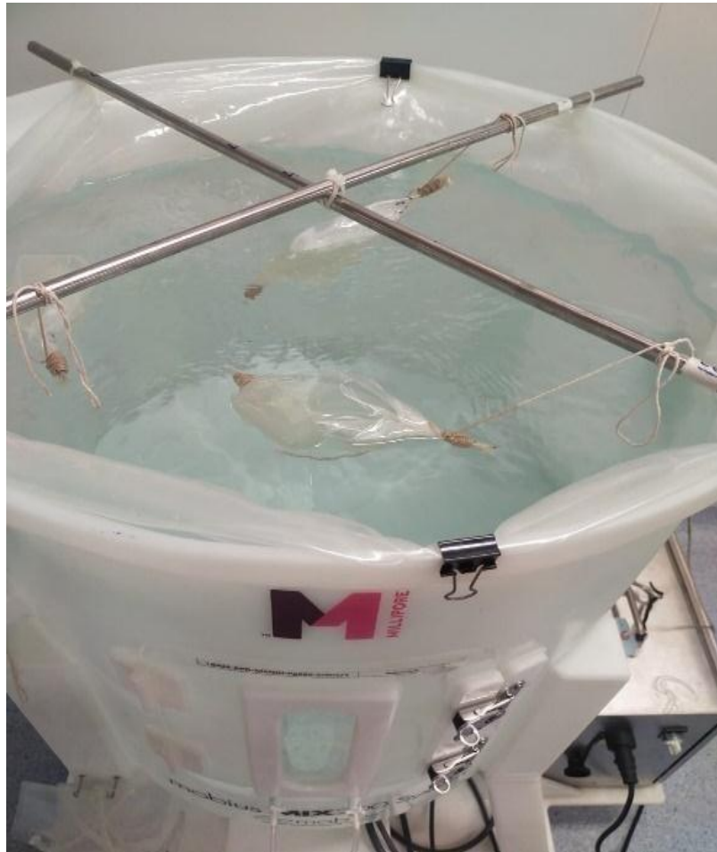
Figure 2.18 Dialysis process against W.F.I for removal of small molecules.
