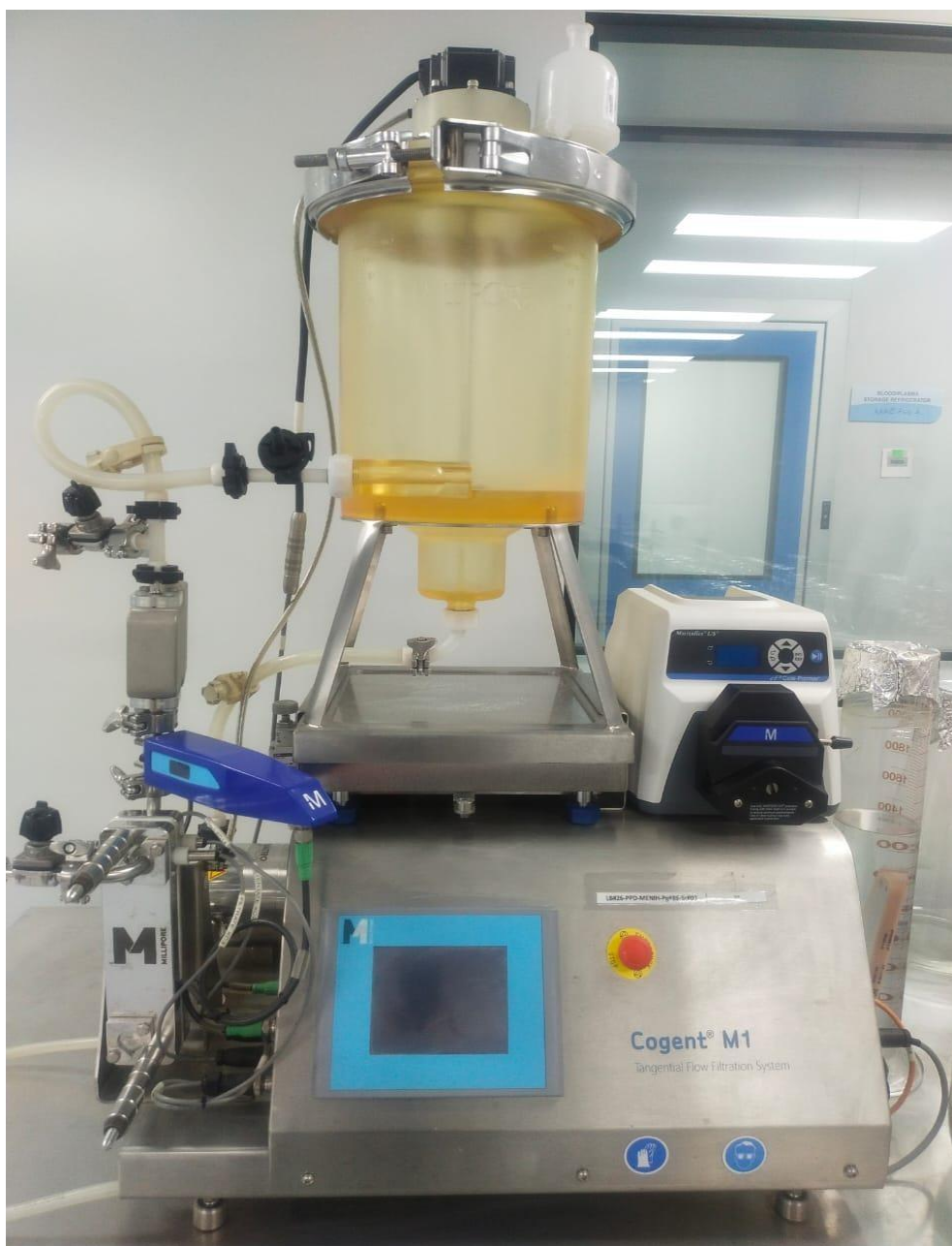
Figure 2.19 TFF for the purification and concentration of immunoglobulins at large scale.
