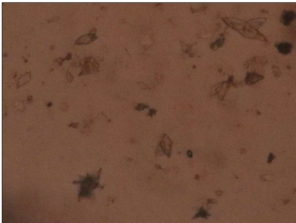
Figure-4.2a: nHap crystals formed by procedure-1; 1000x optical, 15x digital zoom.
