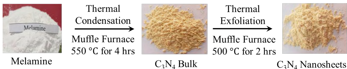
Figure 2.1: Schematics of synthesis of C_3N_4 nanosheets
