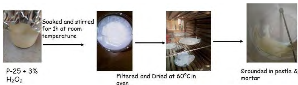
Figure 2.2 : Flow diagram of synthesis of HMT
