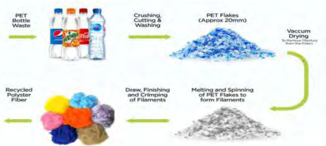
Figure : 2.4 PET bottles recycling processes flowchart.
