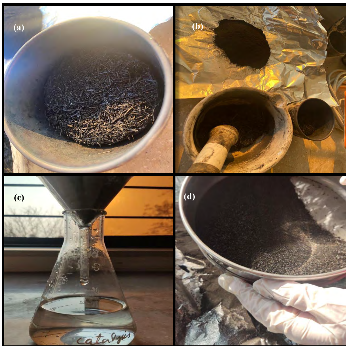
Figure 5: Synthesis of activated carbon from pristine Parthenium . (a) carbonization at 400 °C (b) manual grinding (c) washing with distilled water (d) sieving through 2 mm sieve.
