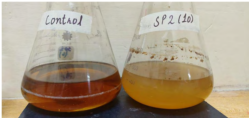
Figure 4.8 Comparison of color of untreated BL and treated BL by bacterial strain SP2 (10) over 168h at 50°C
