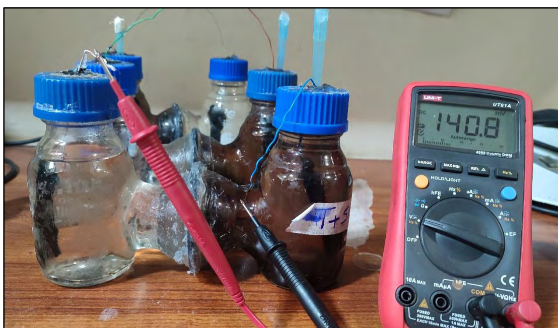
Figure 8: Recording voltage readings using a precision multimeter
