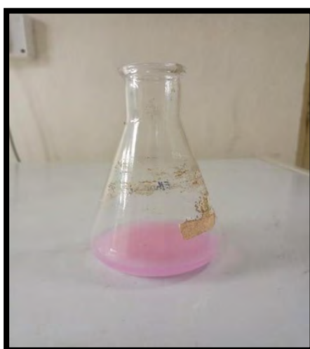
Fig. 4.31. Permanent pink after titration with KOH for FFA content
