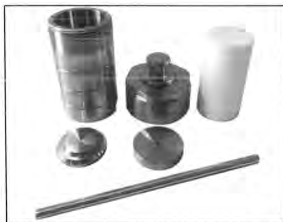
Figure 1- 8 Teflon lined autoclave.
