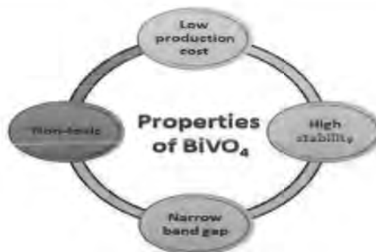
Figure 1.7 Properties/features of \text{BiVO}_4 nanoparticles
