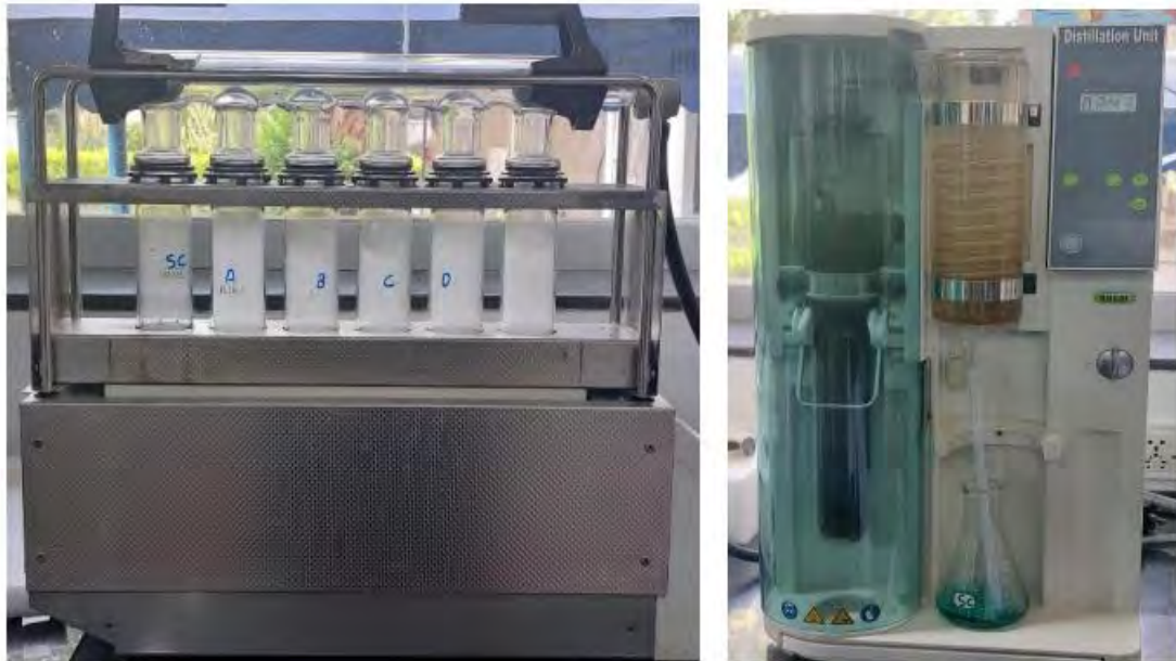
Figure 3.9.2 Kjeldahl System comprising Protein Digestion Apparatus (left) & Distillation Unit (right) at the Institute of Nutrition and Health, Islamabad.
