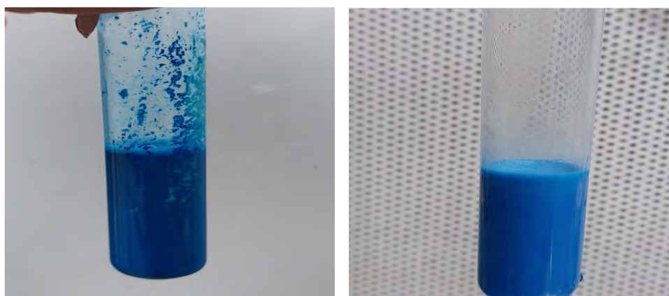
Figure 4.1 Pictorial representation of MDRT, before incubation (left), after 6hours of incubation (right).
