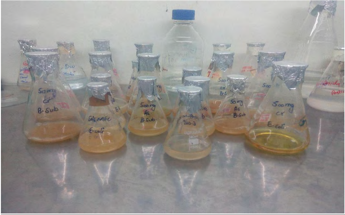
Figure 3.2 Shake flask fermentation setup to check the toxicity of heavy metals via bacterial specimens.
