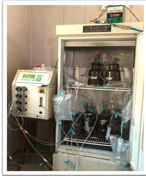
Figure 3.5: Experimental setup for the biogas upgradation with MECs
