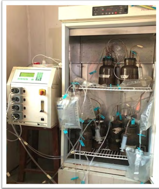
Figure 3.4: Experimental setup for the biogas upgradation without MECs
