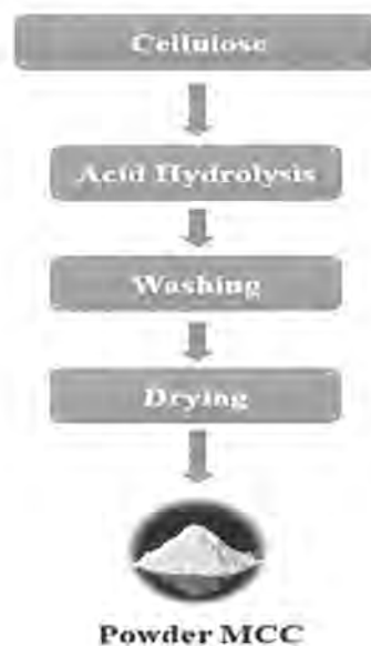
Figure 2.6 Typical procedure for the isolation of MCC from purified cellulose
