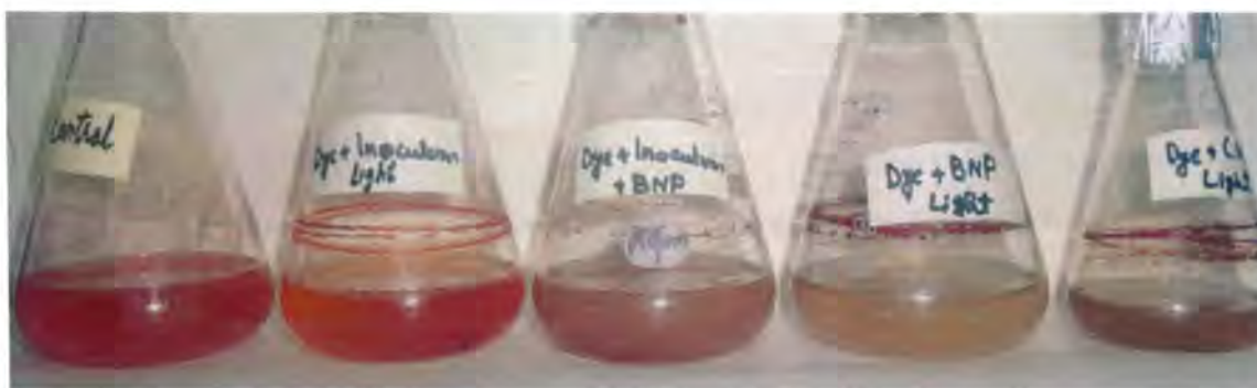
Fig. 4.1: Change in color of AR 151 (50 ppm) by A. niger , A. niger + B Ag 0 NP (100 ppm), B Ag 0 NPS (100 ppm), C Ag 0 NPS (100 ppm).
