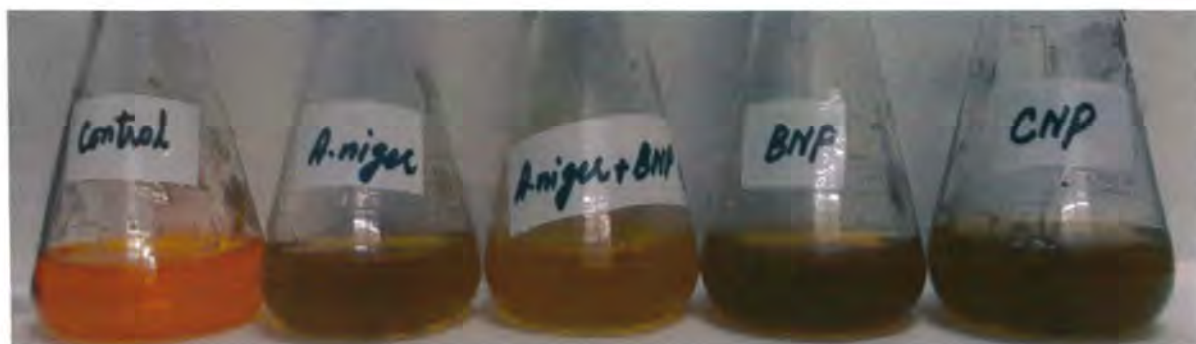
Fig. 4.14: Change in color of Or II (20ppm) by A.niger , A.niger + B Ag 0 NP (100ppm), B Ag 0 NP (100ppm), C Ag 0 NPS (100 ppm).
