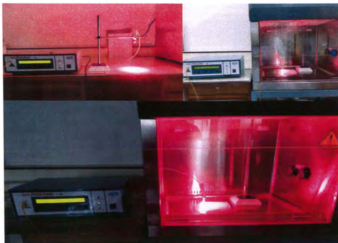
Figure 3-3: A 635\text{nm} diode laser developed by NILOP, Islamabad, is used as a light source
