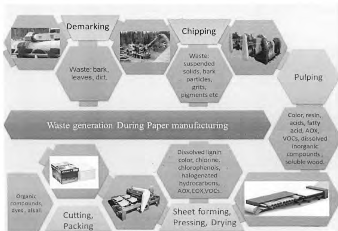
Figure 2. 3 : waste generation During Paper manufacturing at various steps
