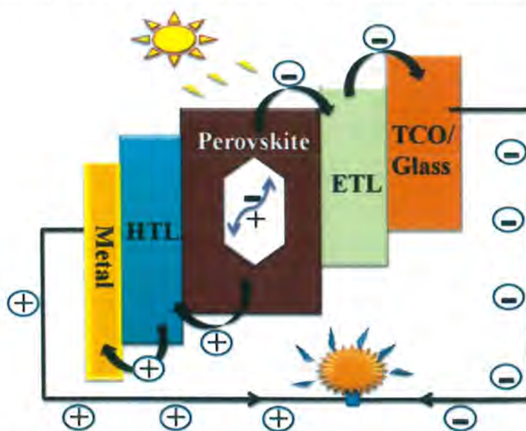
Figure 1.7: The schematic working principle of a perovskite solar cell 63
