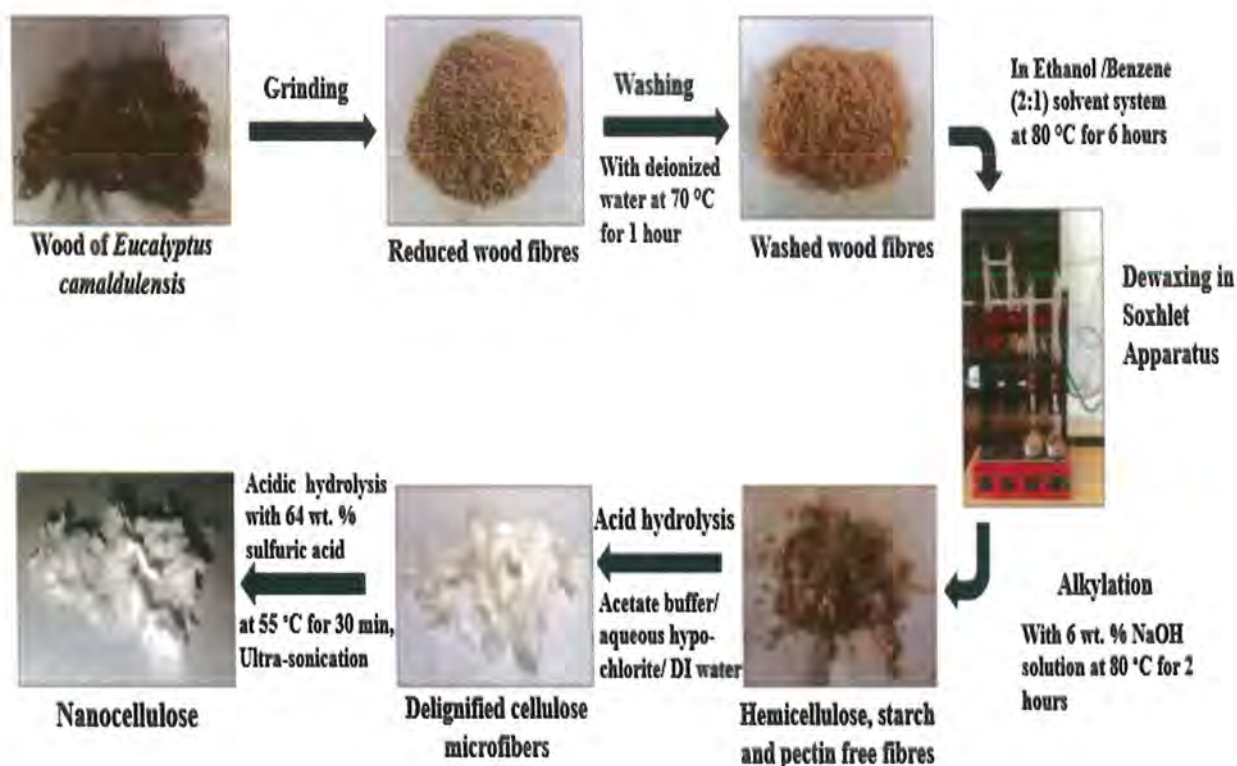
Figure 2.1: Extraction of nanocellulose (NC) from hardwood of Eucalyptus camaldulensis
