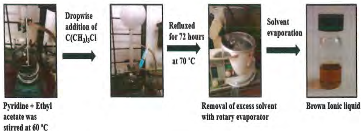
Figure 2.2: Synthetic scheme of tertiary butyl pyridinium chloride ionic liquid (PyIL)
