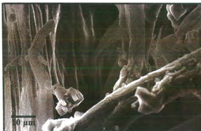
Figure 3.11: SEM micrograph of extracted NC taken at magnification 10 \mu\text{m} .
