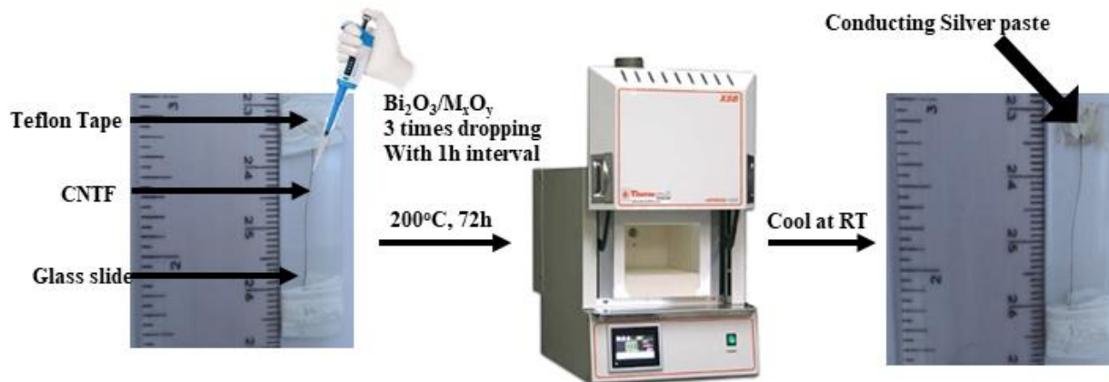
Figure 2.1. The schematic illustration of electrode fabrication
