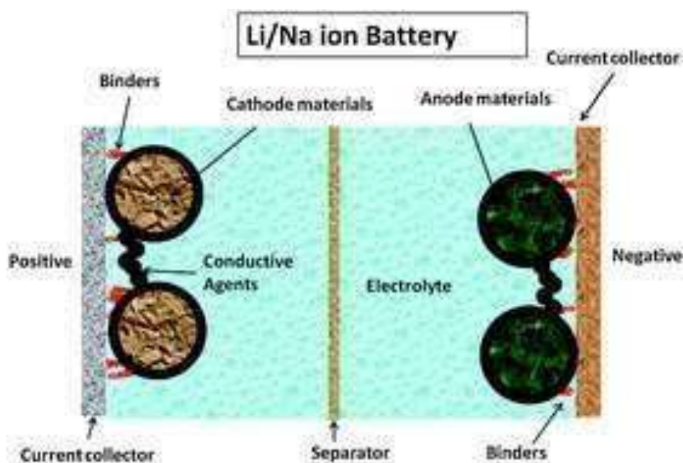
Figure 1.5 Schematic diagram of a battery representing binder adhesion of active particles with current collector 43 .
