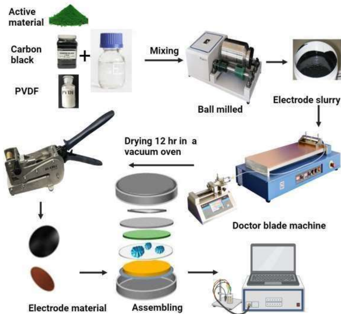
Figure 2.8 Schematic representation of coin cell fabrication
